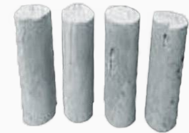
Concrete Cylinders with Sugar Cane Fiber from STI College Muñoz-EDSA aims to encourage recycling by incorporating sugar cane fibers into concrete cylinders and though it is made of biodegradable materials, it is still as strong as the regular concrete
