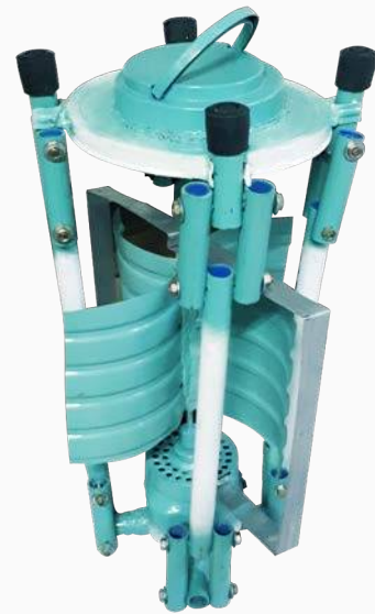
Portable Wind Turbine from STI College Cubao that shows an alternative source of electricity by utilizing wind energy with the case and wind panes were all made from recycled materials
