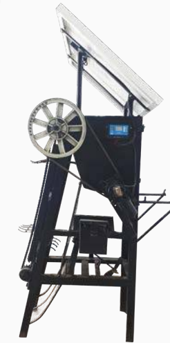
Automatic Canal Waste Collector also from STI College San Fernando that can gather plastic waste from the water systems and runs effectively on solar energy
